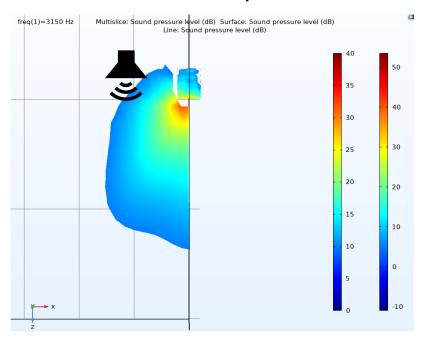
This is the dispersion diagram for a regular system with front firing speakers.
