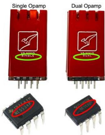
Step 3: Exercise caution while handling opamps, as they are sensitive to polarity. Plugging them in the wrong orientation can result in immediate damage. Identify the pin 1 indicator on the opamp as well as the corresponding half-moon cut on the opamp socket. Before inserting the new opamp, ensure that you have the correct orientation.
