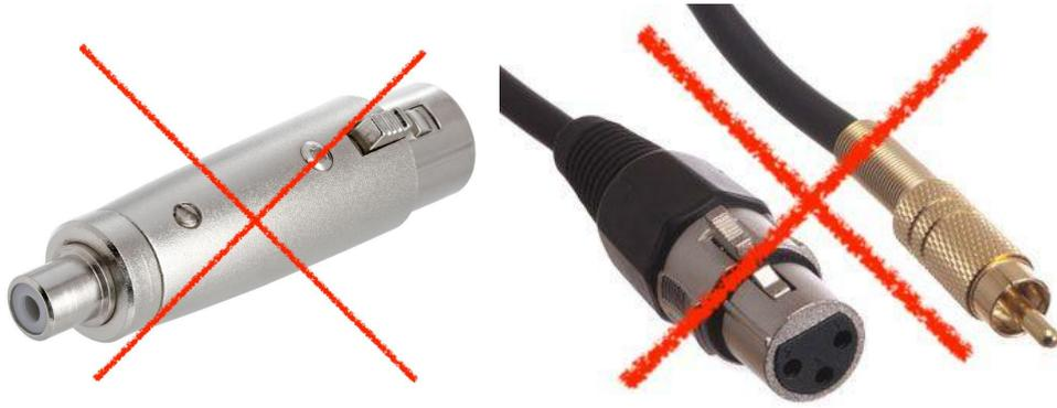
Therefore, please only use the custom made, Burson marked XLR-RCA adapter we have provided in our accessories box to connect the XLR outputs of our products to any downstream amplifiers with RCA inputs.
