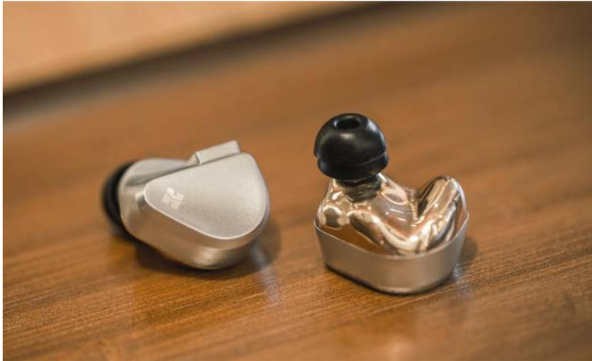
The Svanar ranks among the most stable earphones at any price. HIFIMAN's engineering team incorporated brass in the front chamber while using aluminum alloy in the rear, which places the center of gravity at the pinna, or visible portion of the outer ear. By doing so, both stability and comfort are maximized, even when enjoying extended listening sessions.
